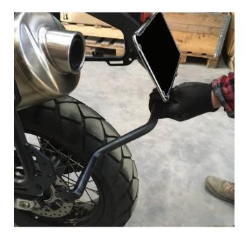
8. Add all four M6 hex bolts, washers and locking nuts. Using a 10mm socket and ratchet on one side while holding down on the other with a 10mm ratchet tighten the bolts and nuts.
