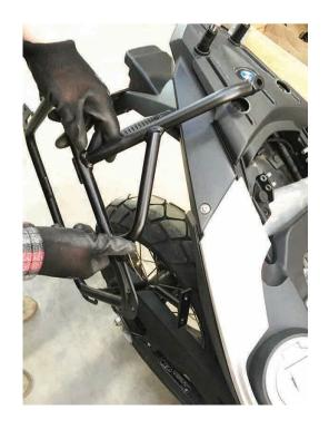
3. Secure it on by using the supplied M8x30mm bolts. Leave it loose.
