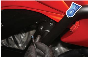
6. Place connector tube between the crash bars. Fasten both sides using four 6x16mm Allen head bolts, washers and nyloc nuts. Use 4mm Allen key and 10mm wrench. Do not fully tighten it, yet.
