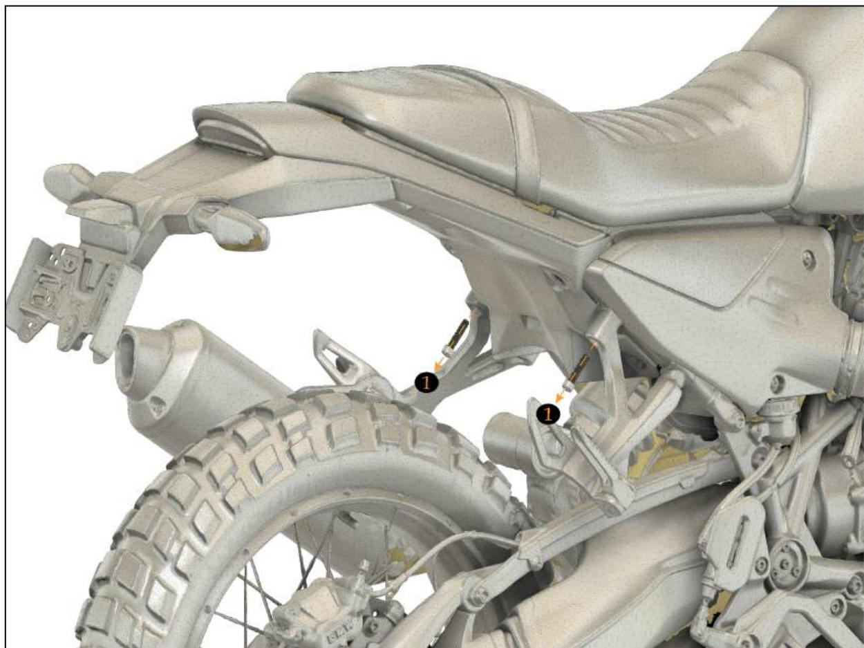
**STEP 2 (Install 34.5mm Spacer + M8 x 60mm Bolt):**
